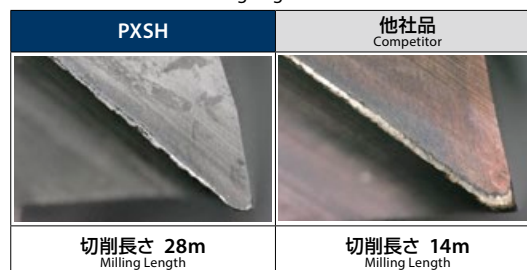
刃先の損傷状態 Wear condition of the cutting edge
