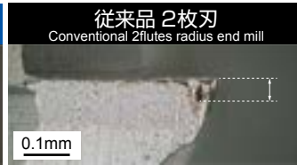
従来品 2枚刃 Conventional 2flutes radius end mill 逃げ面摩耗幅 0.065mm Flank wear
