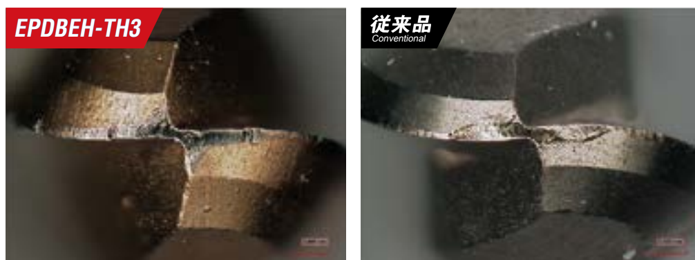
図 60分加工後の摩耗状態 Figure: Wear condition after 60 minutes of machining
