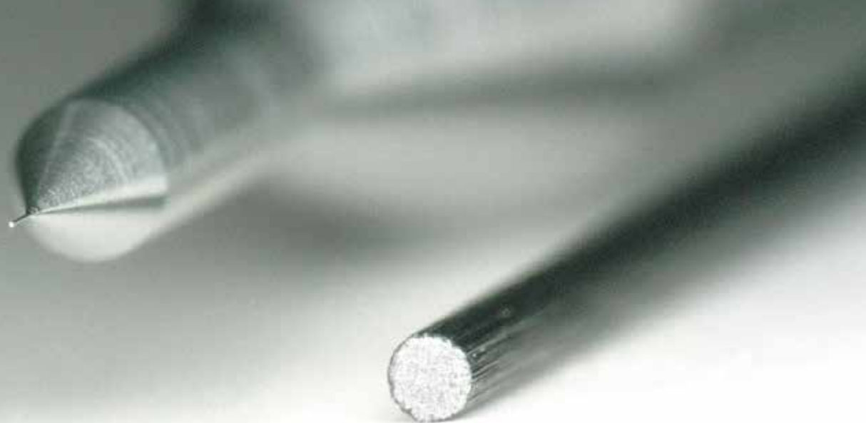
Left : \phi 0.03mm drill cutting tip Right : \phi 0.5mm lead for mechanical pencil
